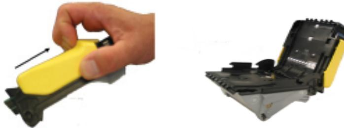
3. Remove the yellow cover from the acceptor module by turning the acceptor module so that the top of the cover is facing you. Wedge the tips of your fingers underneath the left and right front top corners of the yellow cover. Lift the corners out and then back toward you. The cover will be released once it has cleared the back ramps, as shown in the diagram below:
