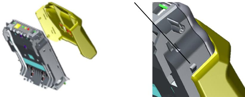
7. Once the yellow cover is in the correct position, move it forward (as though you were opening the acceptor module) until the cover locks into place.
