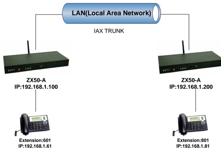
Register the ZX50-A as an peer in ZX50-B(via SIP trunk),so the extensions in ZX50-A can make calls to ZX50-B's extensions via this "special" trunk.
