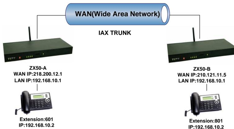
The configuration is same as above guide(7.2 Combine two ZX50 IP PBX in the same network) , but use the public IP address as the "HOST" settings, set as below:
