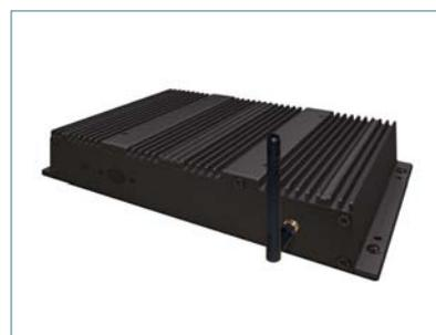
**External wireless antennas boost the performance in connectivity.**
